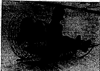
IT'S A BREEZE—Traveling the snow-packed streets of Parsons, Kan., is a breeze with this sled equipped with an "outboard motor." The "outboard" is really just an old washing machine motor and a 16-inch fan. Gayle Marie Coots, 4, is the happy owner of the fan-driven sled, built by her automobile-mechanic father. He has to run to keep up with it.
